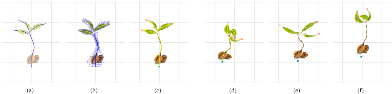
Figure 1: An example deformation image of sprout using our freeform deformation axis (a) original image and a drawn freeform deformation axis (b) a generated mesh according to FDA's thickness value (c) setup of position constraints (d)-(f) shape deformation results
